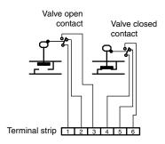
inductive contacts (valve closed) Valve open contact Valve closed contact (red LED) (green LED)
