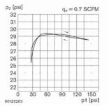
$p_1$  = Supply pressure;  $p_2$  = Secondary pressure; qn = Flow rate
