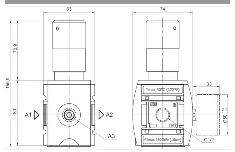
A1 = inputA2 = outputA3 = pressure gauge connection
