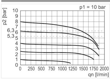
Flow rate characteristic (setting range p2: 0.5 - 10 bar)
