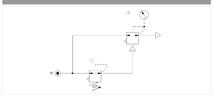
1) precision pressure regulator2) pressure regulator valve, pneumatically operated
