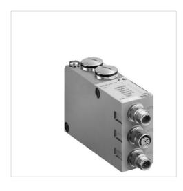
Version Driver 0 ... 50 °C Ambient temperature min./max. Operational voltage electronics 24 V DC Power consumption electronics 0,05 A 24 V DC Operating voltage, actuators Actuator voltage tolerance -10% / +10%
