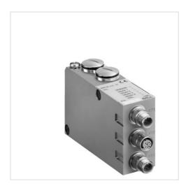
Version Bus coupler with driver 0 ... 50 °C Ambient temperature min./max. 24 V DC Operational voltage electronics -15% / +20% Electronics voltage tolerance Power consumption electronics 0.05 A 24 V DC Operating voltage, actuators Total current for actuators 3 A IP65 Protection class Number of solenoid coils max. 32 Max. power consumption per coil 0,1 mA Generic emission standard in accordance EN 61000-6-4 with norm
