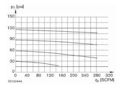
$p_1$  = Supply pressure;  $p_2$  = Secondary pressure;  $q_n$  = Nominal flow
