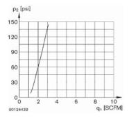
$p_2$  = Secondary pressure;  $q_{n \text{ min.}}$  = Min. nominal flow
